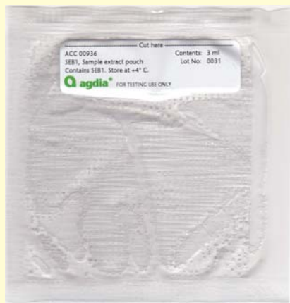
Step 1 Open the ImmunoStrip sample extraction bag.
