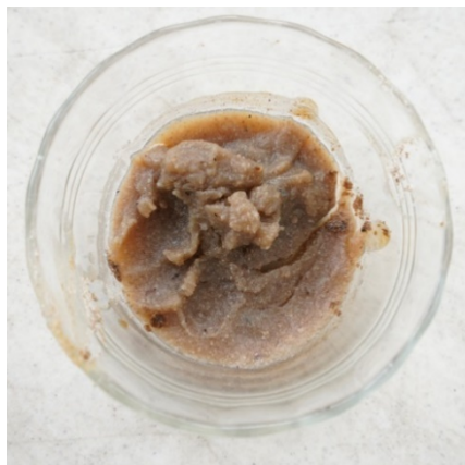
2. Potassium silicates will form a goopy gel when mixed with concentrated fertilizer solutions.
